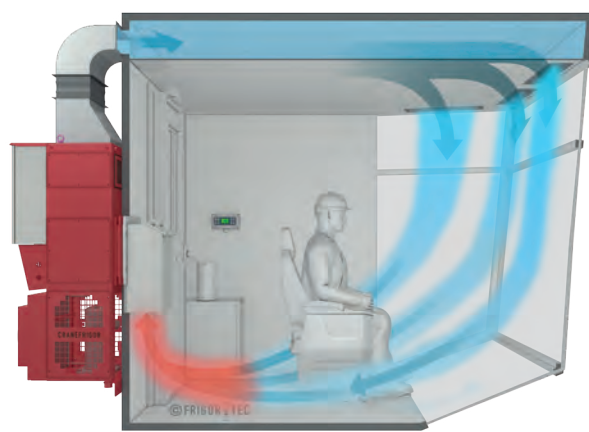
Fig. 3 Procedural principle for crane cabin cooling
