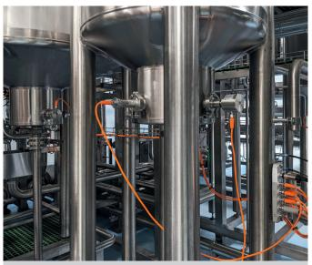
With IO-Link sensors for temperature, turbidity, conductivity, level, flow and pressure, Anderson-Negele can offer almost all measuring ranges from a single source. Thanks to Flex-Hybrid technology, sensors can be operated in digital and analog mode in parallel (IO-Link and 4...20 mA).
