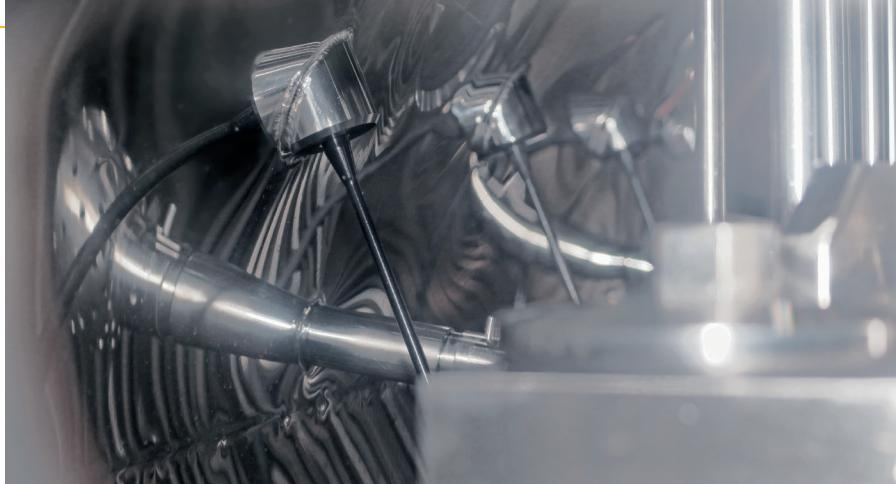
Based on the positive experiences gained, Friesland-Campina has also switched from point level measurement with LS measuring rods of different lengths to continuous level measurement with NSL-F for the dosing unit for dessert creams. For this purpose, the probe (shown on the left picture, top right in the picture) was retrofitted to the container with a weld-on socket. The four LS switches remain installed as redundant system.
